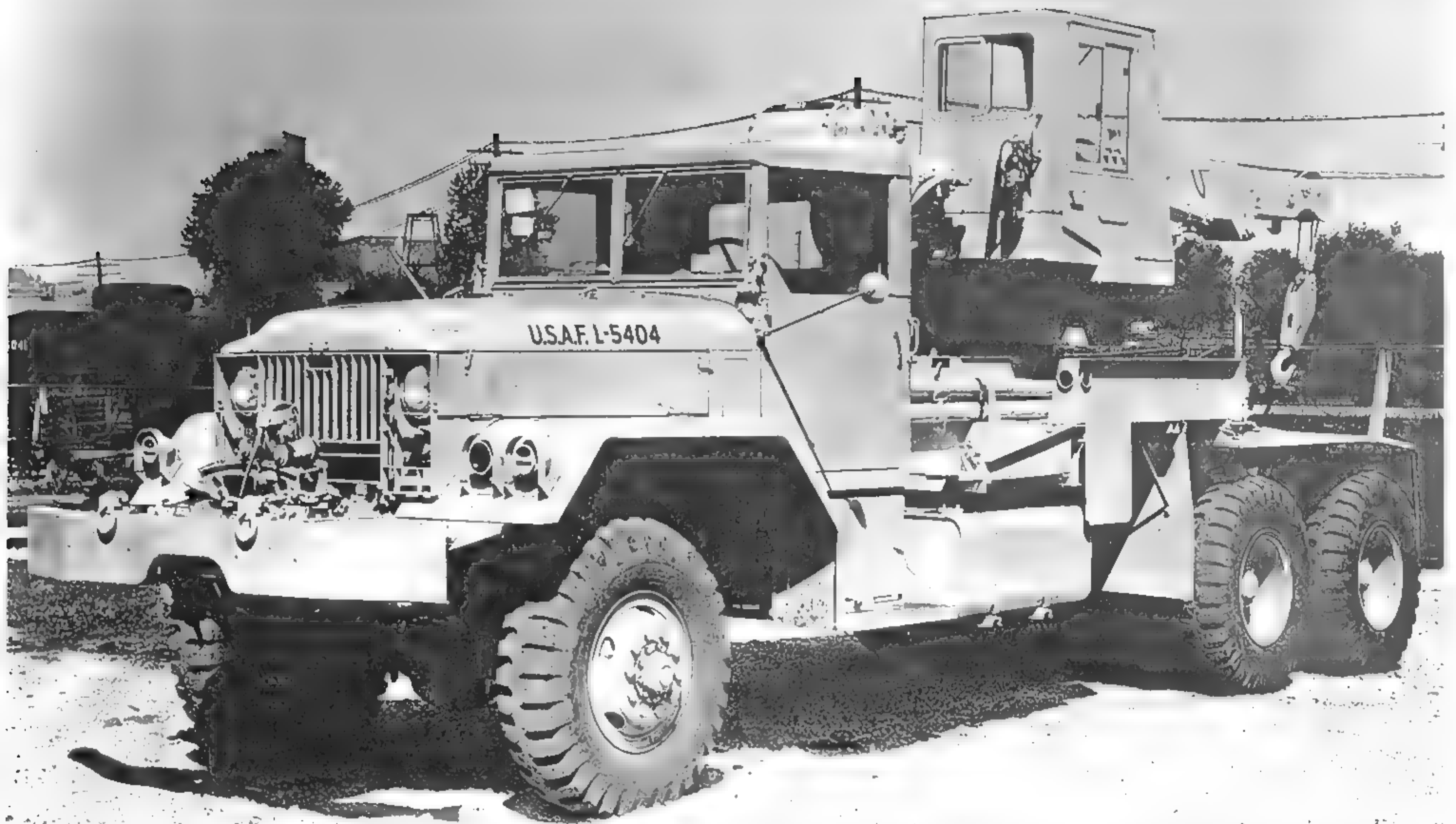
The M246 was a tractor wrecker based on the G-744 chassis. Intended primarily for aircraft recovery, its boom would extend up to 26 ft. and, rather than the rear recovery winch, there was a fifth wheel installed to tow low-bed semi-trailers. The M246 was built on a 215-in.-wheelbase chassis. (Photo courtesy of the Patton Museum).
